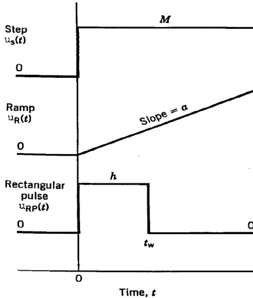
**Figure 5.2.** Three important examples of deterministic inputs.
