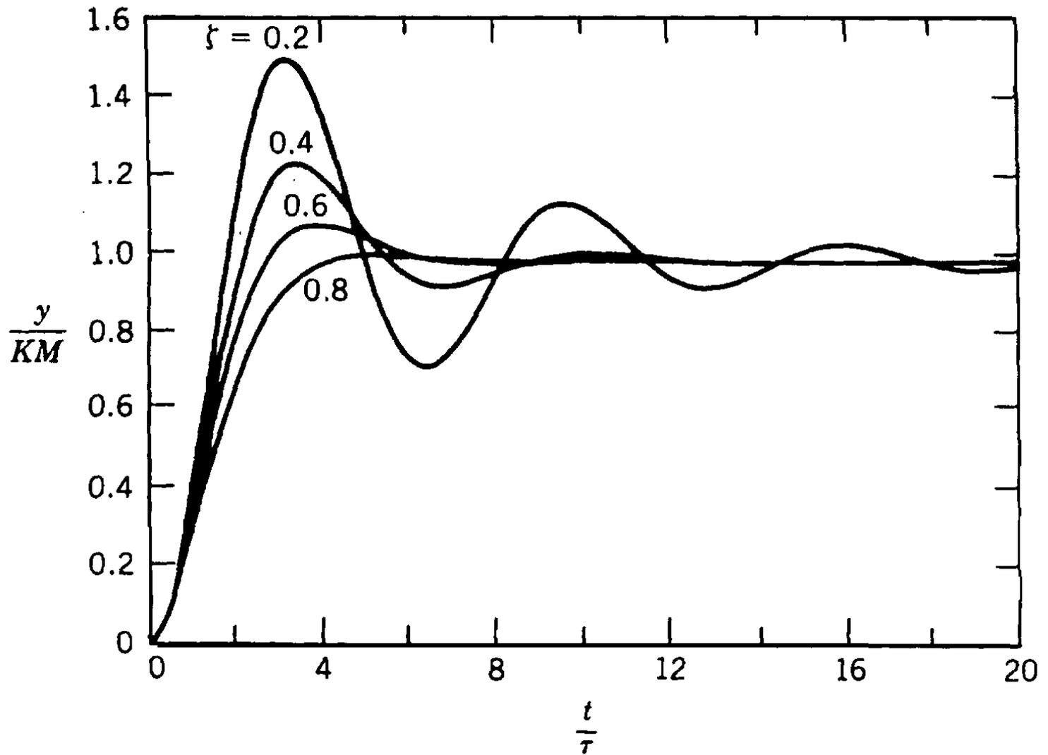
Figure 5.8. Step response of underdamped second-order processes.
