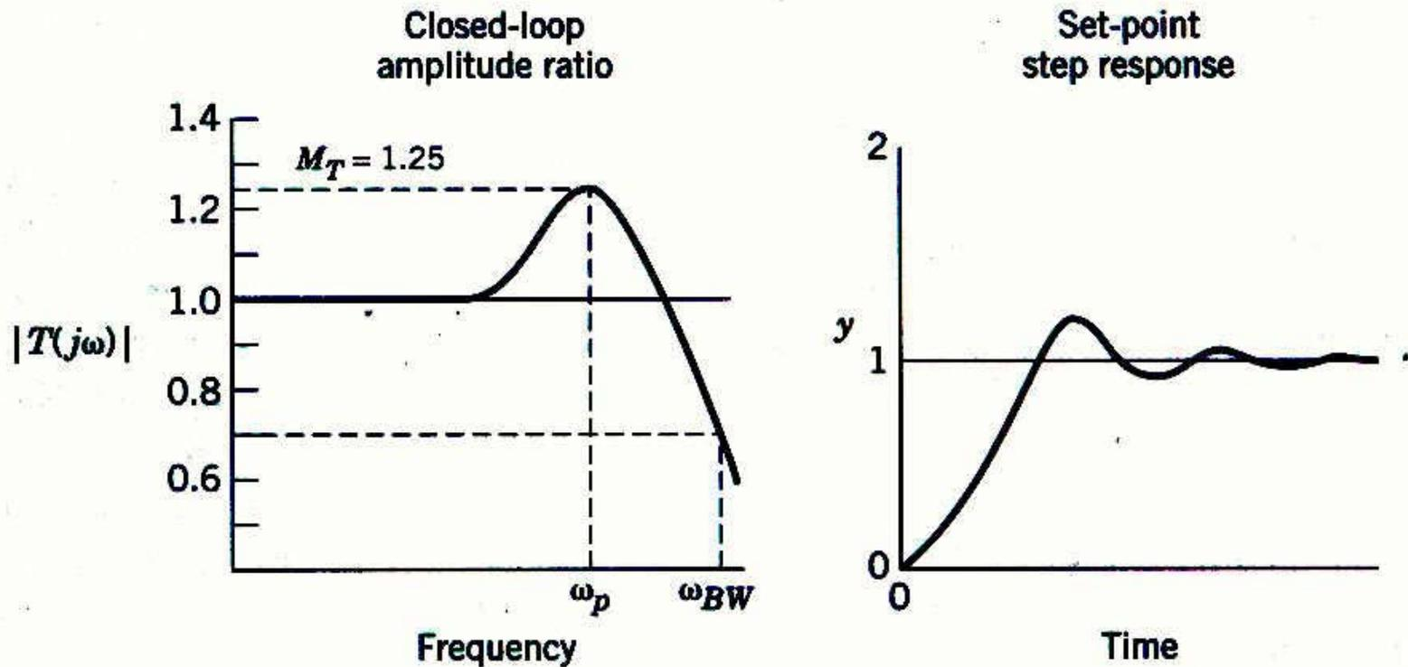
Figure 14.14 Typical closed-loop amplitude ratio  $|T(j\omega)|$  and set-point response.
