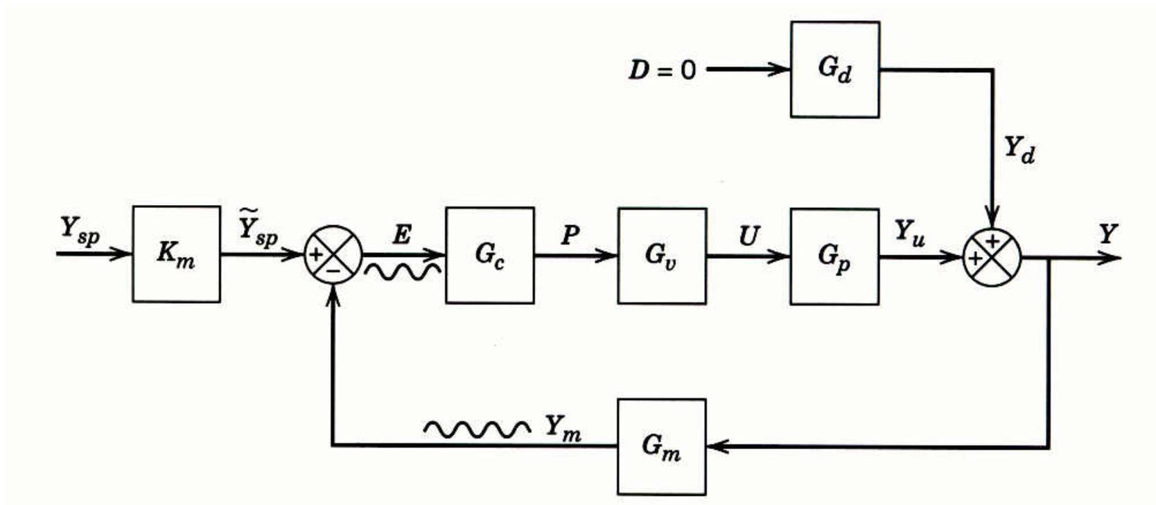
Figure 14.4 Sustained oscillation in a feedback control system.
