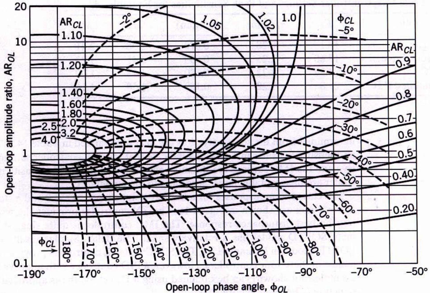
Figure 14.15 A Nichols chart. [The closed-loop amplitude ratio  $AR_{CL}$  (—) and phase angle  $\phi_{CL}$  (---) are shown in families of curves.]
