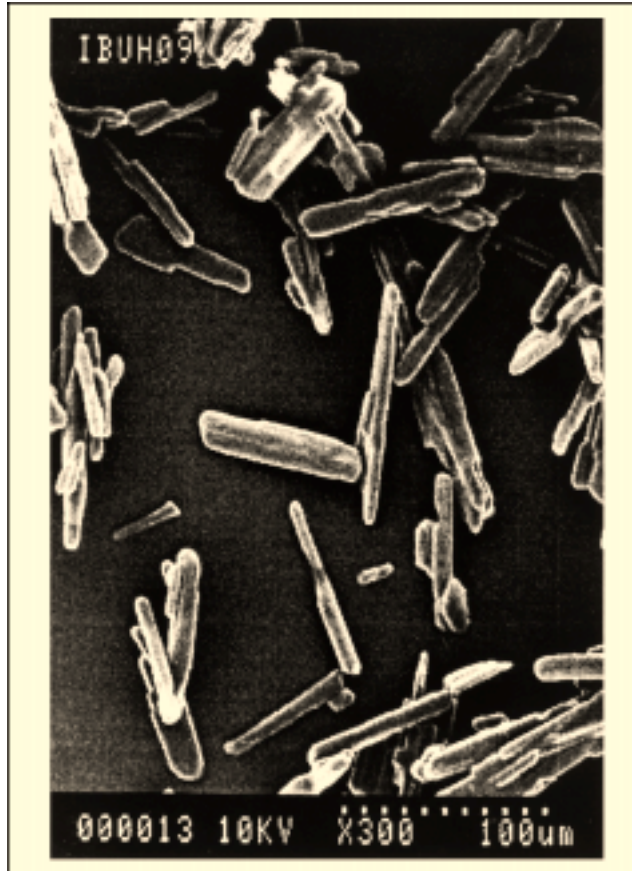
Figure 10. Ibuprofen crystals grown from hexane. Courtesy of Storey (1997).
