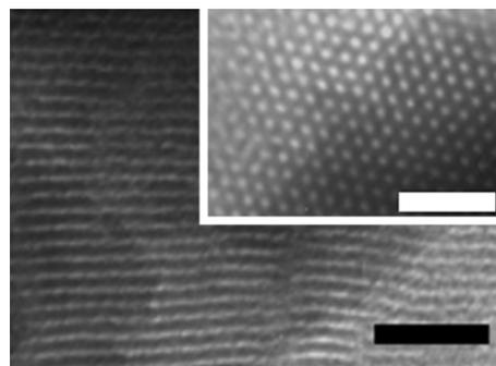
Fig. 1 TEM images of calcined mesostructured silica thin films recorded along the [110] and [100] (inset) zone axes. Both scale bars are 50 nm.
