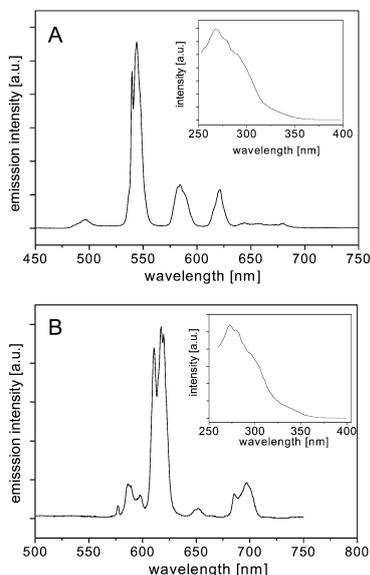
**Fig. 2** PL emission and excitation (insets) spectra of Tb<sup>3+</sup>–phen (A) and Eu<sup>3+</sup>–phen (B) doped mesostructured films (both 2 wt%).
