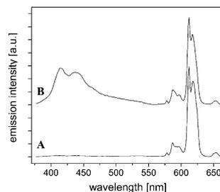
**Fig. 3** PL emission spectra of 6 wt% Eu<sup>3+</sup>–phen complex doped into (A) mesostructured P123/silica and (B) pure silica glass thin films. The emission intensities of the two spectra are normalized with respect to the Eu<sup>3+</sup> crystal field transition <sup>5</sup>D<sub>0</sub>→<sup>7</sup>F<sub>2</sub> at 615 nm.
