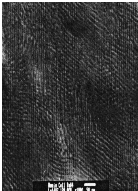
Fig. 6. TEM image of PVAc- g -PS graft copolymer 2c with dark PS-rich domains imbedded in the lighter PVAc matrix. The scale bar represents 50 nm.
