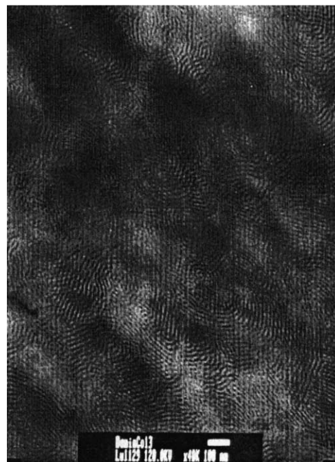
Fig. 5. TEM image of PVAc- g -PDMS graft copolymer 1 with dark PDMS-rich domains imbedded in the lighter PVAc matrix. The scale bar represents 100 nm.
