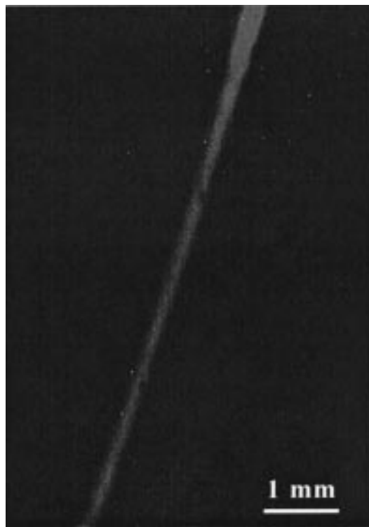
Figure 4. Polarization image of calcined 3D hexagonal mesoporous silica fibers prepared using \text{EO}_{106}\text{PO}_{70}\text{EO}_{106} . The fiber axis is oriented 45^\circ with respect to the upper and lower polarizers.
