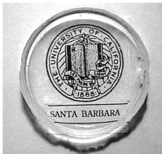
Figure 1. A mesostructurally ordered transparent block copolymer/silica monolith, prepared with a composition of 62 wt % EO 106 –PO 70 –EO 106 . The monolithic disk is 2.5 cm in diameter and 3 mm thick.
