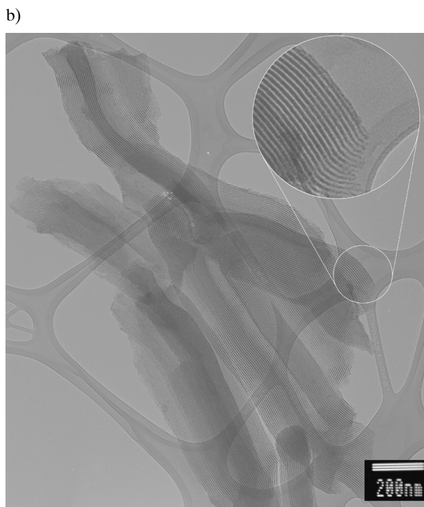
Fig. 2. Representative TEM images of mesoporous silica prepared at pH 1.2 in the presence of small amounts of fluoride. a) Entire cross-section of a single silica fiber. The nanochannels are arranged on a 2-D hexagonal lattice. b) Image of nanochannels extending over several hundred nanometers and following the fiber's curvature with high fidelity. Inset: Magnification of a selected area, demonstrating the ordered channel structure. c) Single +\pi -disclination defect. TEM micrographs were obtained with a 2000 JEOL transmission electron microscope (200 kV).
