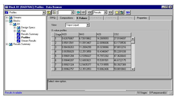
The K-value for NH3 on stage 1 is 6.73. These results demonstrate that when you use apparent components, Aspen Plus also reports the K-values calculated by RadFrac (or any flash) on an apparent basis.
