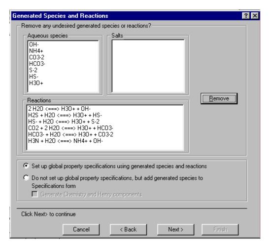
**Note** Any time you know that a reaction can be neglected because of expected process conditions, you should remove it from the solution chemistry, to decrease the execution time required for your simulation.
