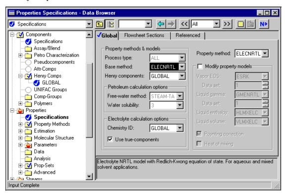
The Electrolyte-NRTL activity coefficient model, ELECNRTL, is the recommended option set for simulations with electrolytes. ELECNRTL calculates liquid phase properties from the Electrolyte-NRTL activity coefficient model. Vapor phase properties are calculated from the Redlich-Kwong equation of state.
