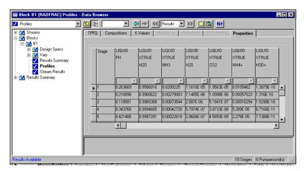
Consider the results for Stage 1. The true composition of NH3 and NH4+ sum to 0.03147 on Stage 1. This value is slightly different from the apparent mole fraction of NH3 reported on the Compositions sheet: 0.03138. This slight difference is caused by the solution chemistry.
