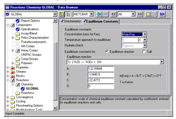
The Aspen Plus reactions database contains over 600 reactions, which cover virtually all common electrolyte applications.
